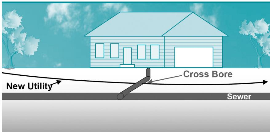
Sometimes the gas pipeline serving a house is accidentally installed so that it crosses through the sewer pipeline. This is called a cross bore, which may occur when trenchless technology is used to install gas pipelines or when sewer lines were not mapped or installed with locatable technology.
