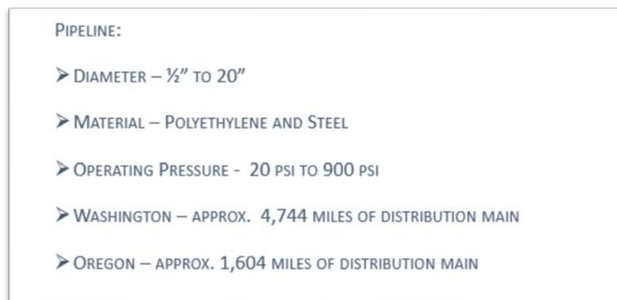
Figure 9-3: Cascade System Pipeline Overview
